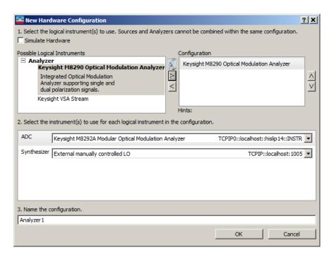
4 In the ADC selection, click on the down arrow and select the desired instrument.
