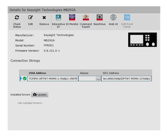
6 Verify that the instrument details shown in the Connection Expert are correct and that the instrument is listed with a green check mark in the "My Instruments" section. If so, the instrument is ready to be connected to the Keysight OMA Software as described in the following section.
