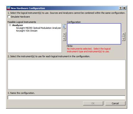
3 From the Possible Logical Instruments list, select Keysight M8290 Optical Modulation Analyzer then click on the ▶ button to add it to the Configuration list.
