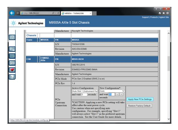
4 If the "Active Configuration" shows a wait time below 15 seconds, select "Auto" in the "New Configuration" list and enter 15 seconds as the wait time. Then press "Apply New PCIe Settings".
