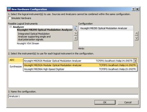
5 In the **Synthesizer** selection, click on the down arrow and select the LO configuration (internal or external LO). With the **M8296A** only an **external manually controlled LO** is supported. This setting can also be used if the test setup does not actually include an LO.
