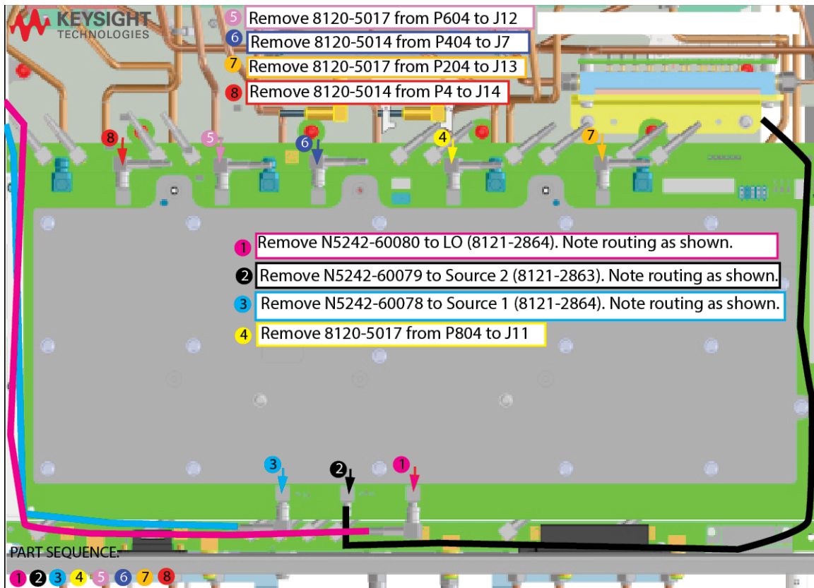
Figure 7-31 Version 6 Synthesizers: A70/A75 LFE Board Remove Cables (8120-5014 (x2), 8120-5017 (x3), N5242-60078, N5242-60079, N5242-60080). (4-port is shown. 2-ports have less cables to be removed. Process is similar.)
