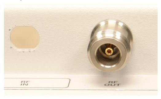
3. Slip the lock- washer and nut over the back of the Type-N connector behind the cover, (2190-0104 item 5 and 2950-0132 item 6 on the parts list). From the rear of the cover, using a 9/16 inch wrench, tighten the nut on the lock-washer and Type-N connector to 35 inch-pounds.
