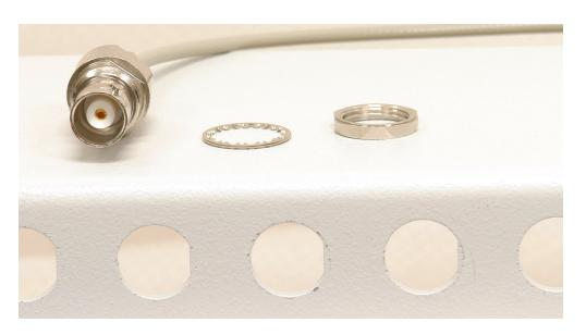
2. Insert the cable end of a BNC connector assembly through a BNC mounting hole so that the BNC connector mounts from the front of the cover (8121-2461, parts list item 8).
