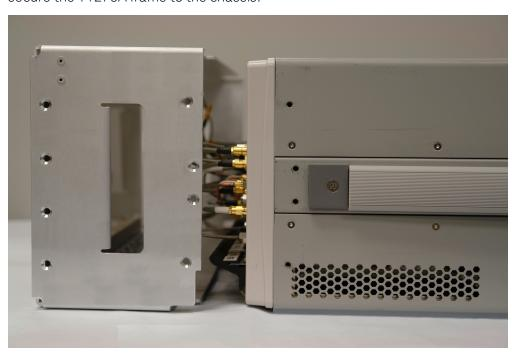
2. Slide the Y1270A frame onto the chassis using great care not to pinch the cables running between the Y1270A frame, and the chassis.
