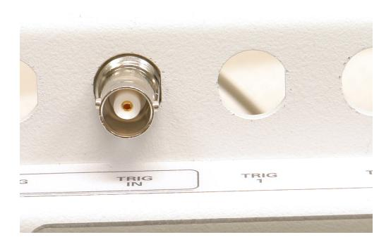
3. Slip the lock-washer and nut over the threaded portion of the BNC connector protruding through the front of the cover (2190-0102 item 9 and 0590-1251
