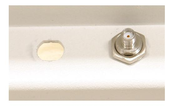
4. Connect a cable (E6630-60004, parts list item 7) to the back side of the Type-N connector and tighten it with a 5/16 wrench to 10 inch-pounds.
