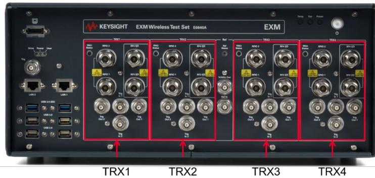
Figure 1. Configure your EXM with 1 to 4 transceivers (TRX)
