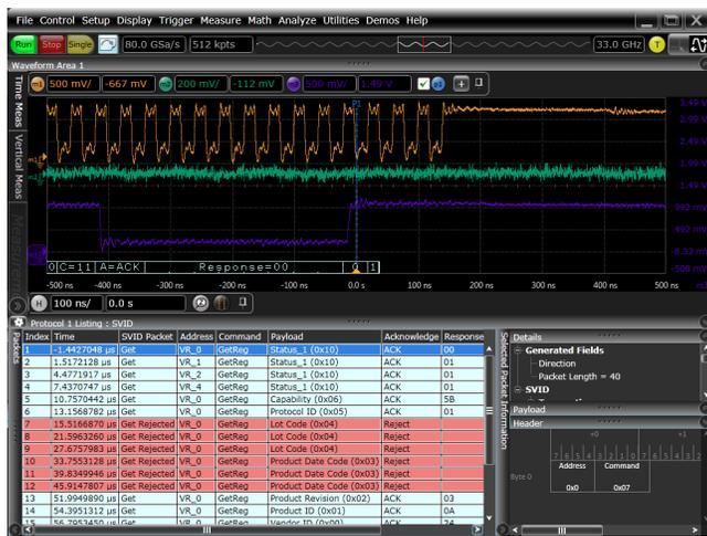
Quickly move between physical and protocol layer information using the time-correlated tracing marker. Display protocol content using embedded decode in the waveform area. Or, see protocol events in a compact listing format. View the decode information in symbols or packets type.
