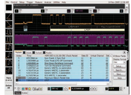
Trigger on and decode MIPI packets.
