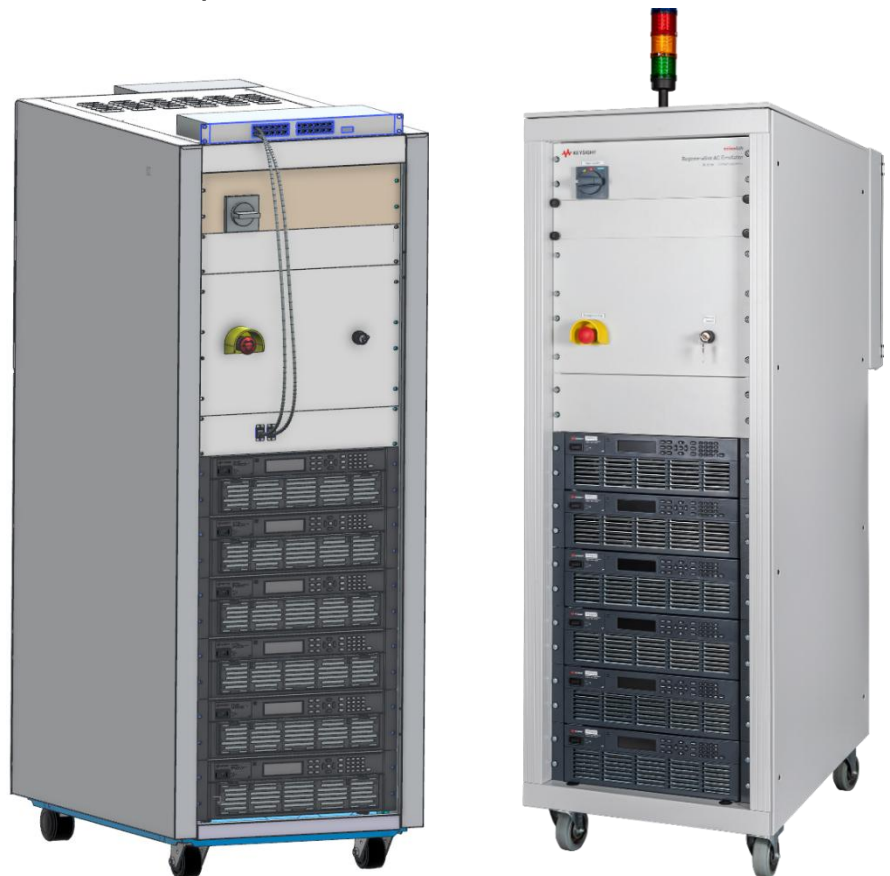
Figure 1. Rendition of SL1215A with high-speed interface for low-latency PHIL grid simulation (left), next to an actual SL1215A (right)
