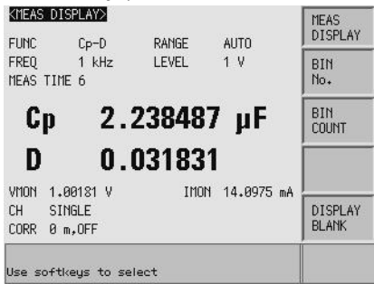
Figure 3-13 Measurement result display screen (when primary parameter is Cp and secondary parameter is D)
