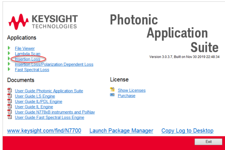
Figure 5 The Launch Pad gives you access to the installed components. Click on "Insertion Loss" to start the wavelength-swept Insertion Loss Engine.
