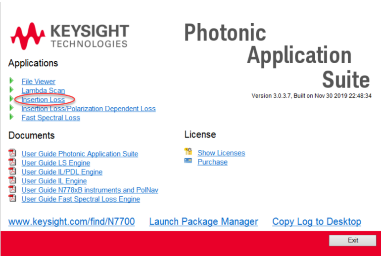
Figure 2 The Launch Pad gives you access to the installed components. Click on “Insertion Loss” to start the Insertion Loss Engine
