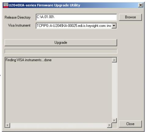
Note: Make sure the U2040 X-Series power sensor is connected to the USB port (or LAN connection for U2049XA) and detected by IO Libraries.
