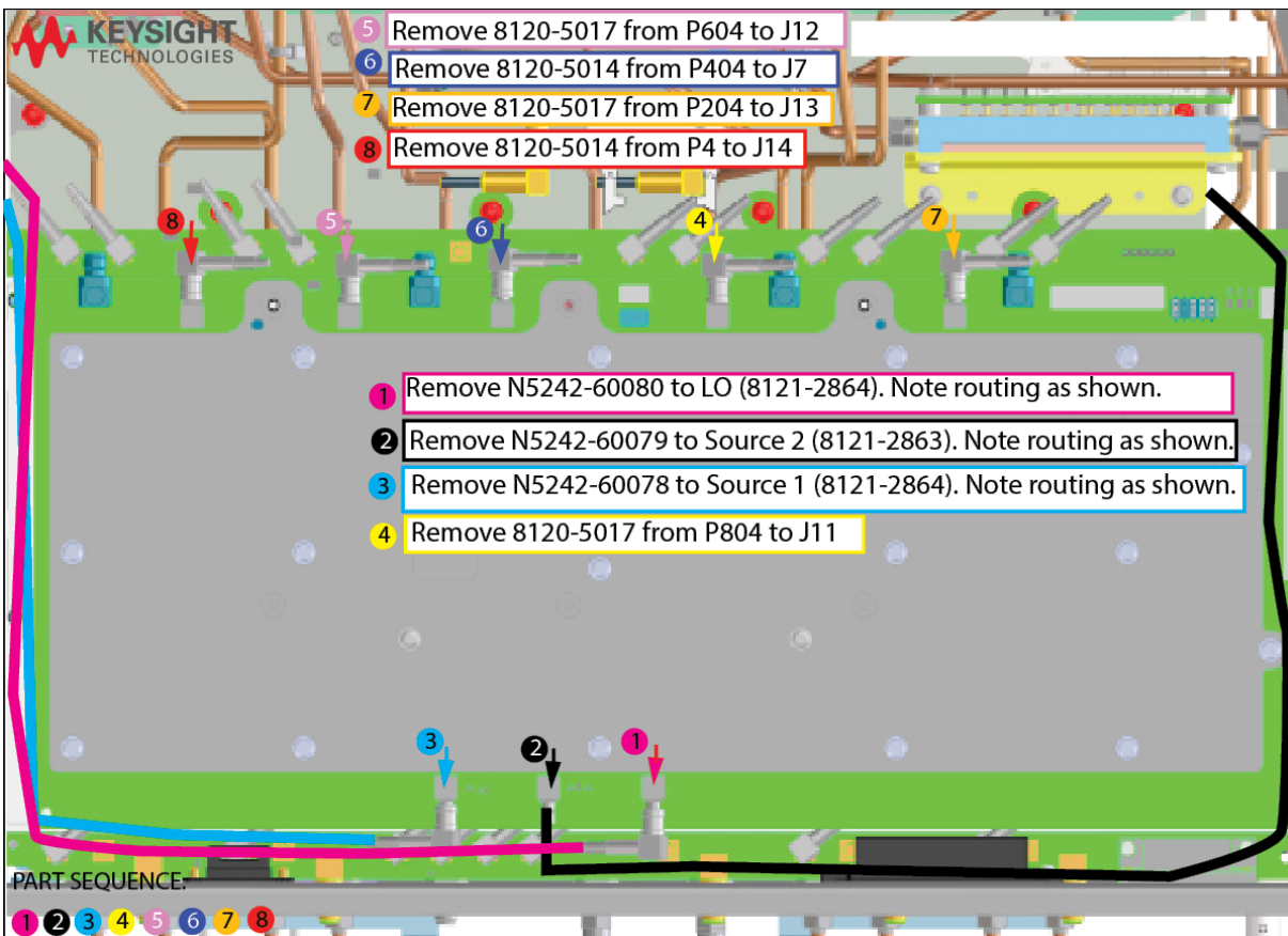
Figure 7-30 Version 6 Synthesizers: A70 LFE Board Remove Cables (8120-5014 (x2), 8120-5017 (x3), N5242-60078, N5242-60080). 4-Port is Shown. 2-Ports are Similar, but with Less Cables.
