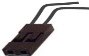
Figure 2 1x2 Header Receptacle with wires
