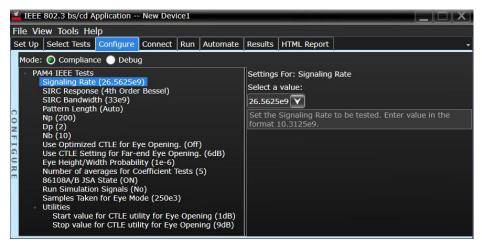
Customize parameters that are specific to your setup, such as signaling rate and CTLE setting. Use default values or enter your own settings including number of waveforms taken, type of pattern, and pattern symbol length. Choose Normal mode to test within limits or choose Debug mode to test to your custom limits and adjust other test parameters. Choose Your Tests
