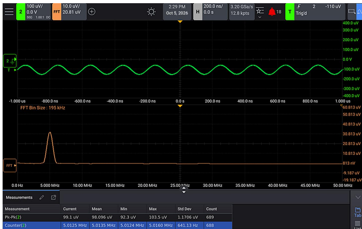
Figure 5. Digital trigger enabling the XR3 to trigger and display a 100 µV sine wave.
