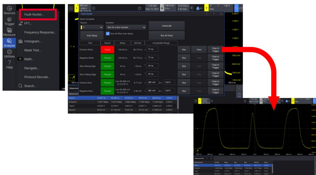
Figure 11. Fault Hunter tests signal characteristics against defined criteria, speeding up debug.
