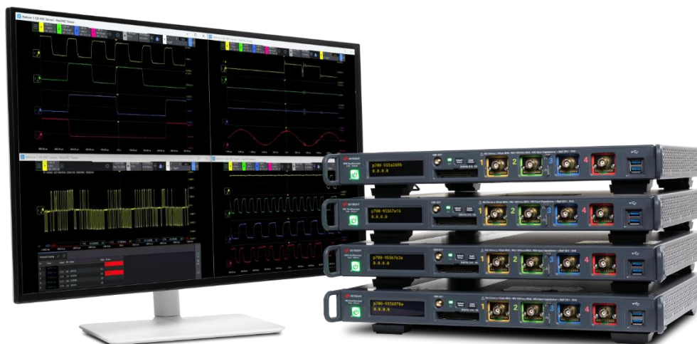
Figure 13. Four XR3s synchronized, running the native InfiniiVision software.
