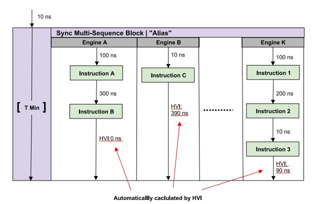
NOTE: Keysight M3xxxA Instruments have an FPGA clock period equal to 10 ns
