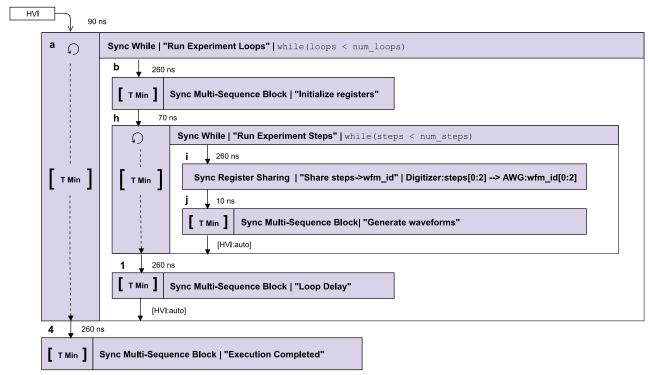
NOTE: 10 ns is the FPGA clock period for M3xxxA instruments
