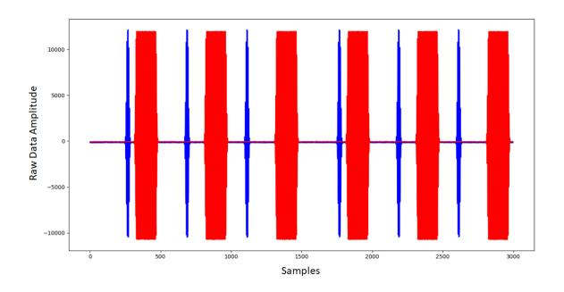
Users can change the experiment parameters to achieve different types of DUT characterization. By setting the experiment parameter  $T2\_flag = 1$ , the Python code execution generates at each experiment step two consecutive I-Q pulses output from AWG CH1 and CH2. The two pulses are separated by a delay tau that increments at each iterations step, whereas the readout delay with respect to the I-Q readout pulses output by the AWG CH3 and CH4 stays fixed.
