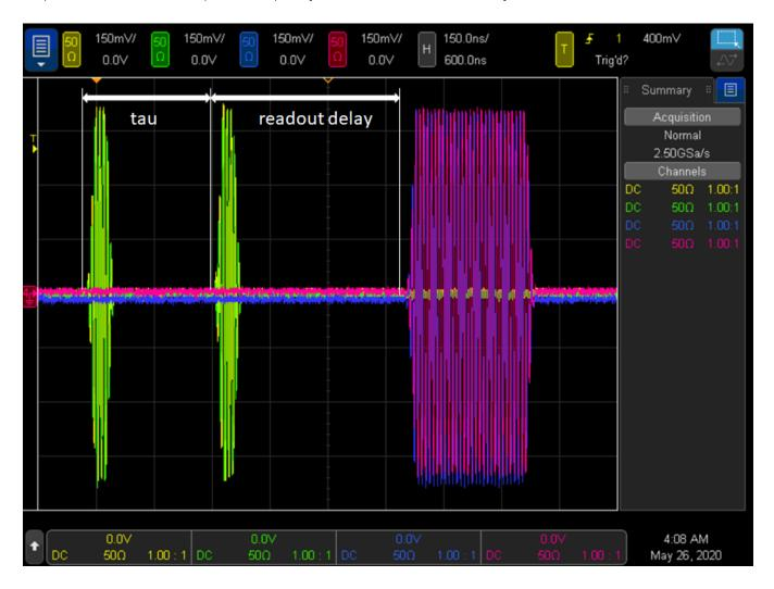
The activation of the T2\_flag parameters allows you to run this programming example to perform an experiment typically used for the characterization of the T2 time, i.e. dephasing time of quantum bits. This experiment is also known as Ramsey experiment. The oscilloscope measurements below represent three iteration steps of such Ramsey experiment.
