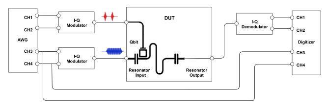
The arbitrary waveforms loaded to the AWG RAM in this programming example include the pi and pi/2 gaussian pulses typically used as Qbit excitation signals. The measurement results included in this document show I-Q pulses output from the AWG channels to produce the typical saturation and readout pulses to be sent to a superconductive Qbit and its resonator to perform the Qbit coherence time T1 (also known as energy relaxation time) and the Qbit dephasing time T2.
