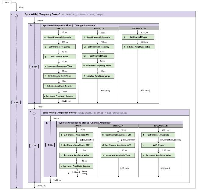
NOTE: Keysight M3xxx Instruments have an FPGA clock period equal to 10 ns NOTE: Keysight M5xxx Instruments have an FPGA clock period equal to 3.33.. ns
