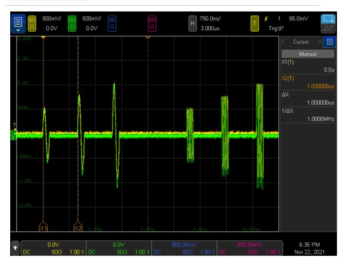
By executing a channel phase reset from HVI, we can ensure that all AWGs included in the application are precisely synchronized and in-phase. In this example measurement the channel phase is also set to start from 0 degrees, however any other arbitrary value can be set. The duration of each RF pulse is set in the Python code to 200 ns. The duration of the amplitude sweep is set to 1 us, which is the time elapsed between two subsequent RF pulses with the same frequency value.
