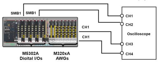
A photograph of the measurement setup used for the measurement results reported in this programming example is also reported below:
