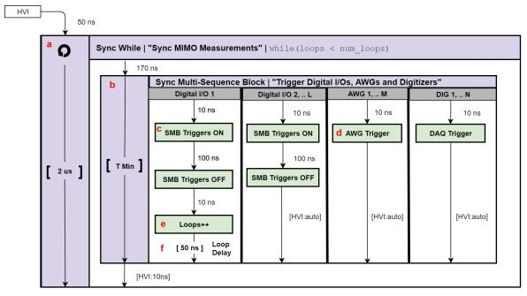
NOTE: Keysight M3xxxA Instruments have an FPGA clock period equal to 10 ns
