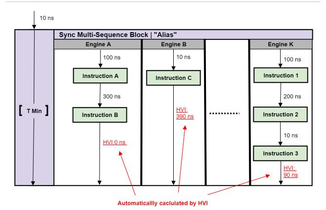
NOTE: Keysight M3xxxA Instruments have an FPGA clock period equal to 10 ns NOTE: Keysight M5xxxA Instruments have an FPGA clock period equal to 10/3 ns
