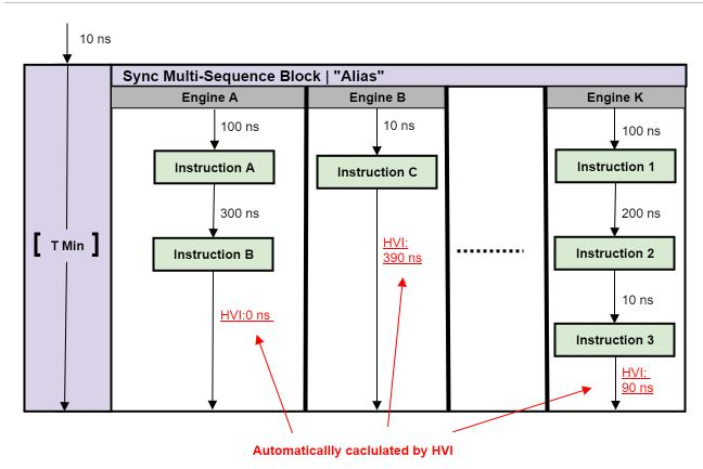
NOTE: Keysight M3xxxA Instruments have an FPGA clock period equal to 10 ns
