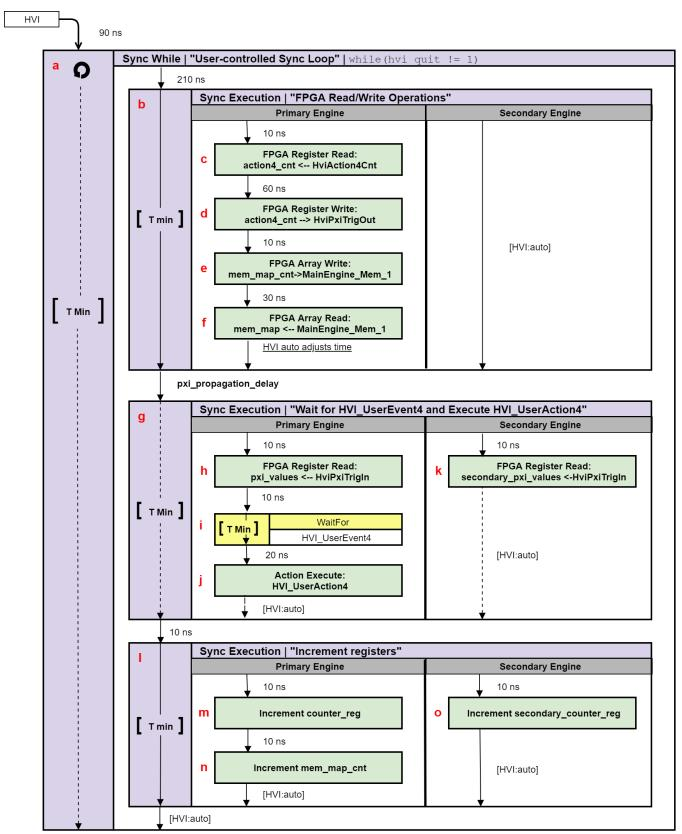
NOTE: 10 ns is the FPGA clock period for M3xxxA instruments
