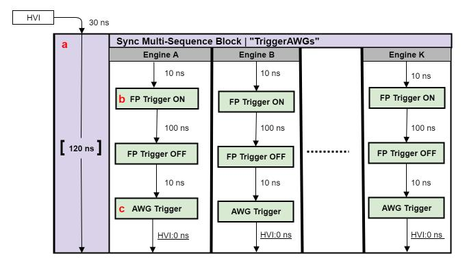
NOTE: Keysight M3xxxA Instruments have an FPGA clock period equal to 10 ns
