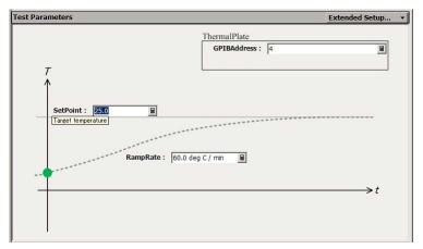
5. Create a test setup for setting up the wait time and the temperature monitor.
