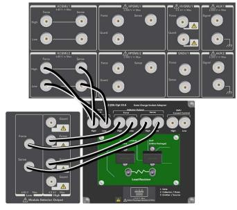
Figure 3-9 Connection Example for High Current Gate Charge Measurement
