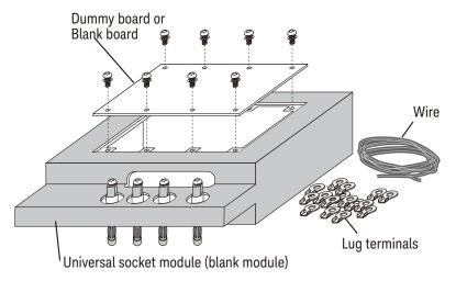
To use this module, see the following simple instruction. For the dimensions and screw holes of a blank board, see Figure 3-32. You can use their handmade socket modules with the same manner as the 3-pin Inline Package Socket Module. See "3-pin Inline Package Socket Module (supplied with the N1273A)" on page 3-93.
