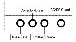
8. Connect the other end of the cables to the terminals on the back side of the socket board.
