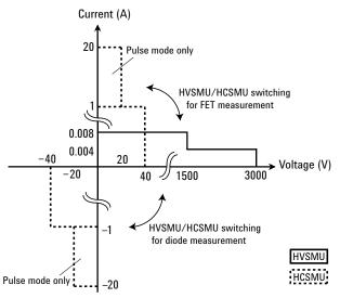
For the GaN current collapse measurement, HVSMU applies high voltage stress to the device under test (DUT) when it is in the OFF state. After that, HVSMU performs voltage measurement and HCSMU performs I-V measurement to monitor the ON state characteristics which is given by the voltage measured by HVSMU and the total current measured by HCSMU and HVSMU.
