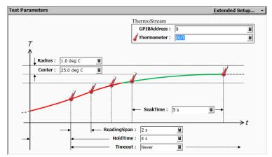
6. Create a test setup for measurement.
