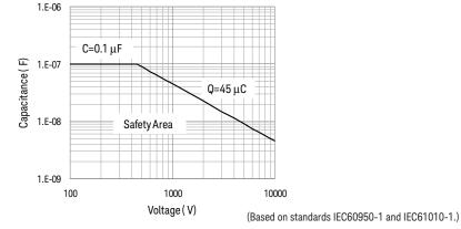
This graph shows the load capacitance vs voltage characteristics generally considered as safety. Use the instrument within the safety area up to 0.1  $\mu$ F or 45  $\mu$ C according to the voltage. Also do not connect the capacitive load over the maximum load capacitance specified for the instrument, for example 10 nF for HVSMU and 5 nF for UHVU.
