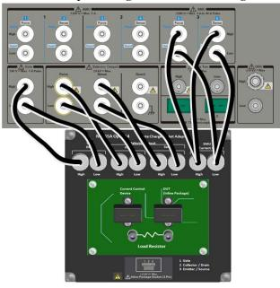
Figure 3-17 Connection Example for High Voltage Gate Charge Measurement
