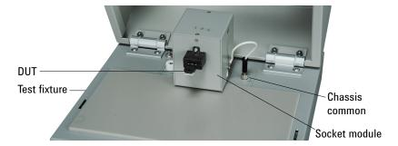
A short plate is furnished with the socket module. It is used for performing the short correction before the capacitance measurement. Set it on the socket before the short correction and remove it after the correction.
