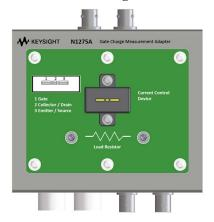
To perform the gate charge measurement, a current control device or a load resistor must be mounted on the socket or the studs.
