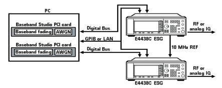
Dual channel fading requires two N5101A Baseband Studio PCI cards and two GPIO brackets.
