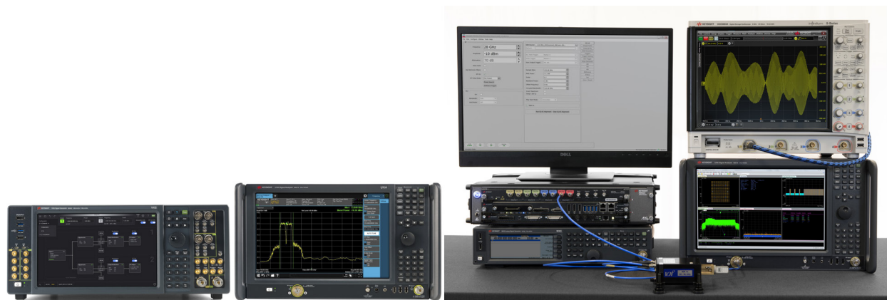
Figure 3. An example of a 5G test bed configuration to enable signal generation and analysis of signals between 50 GHz and 110 GHz with wide bandwidths up to 5 GHz
