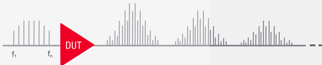
A multi-tone signal into an amplifier produces many complex mixing products
