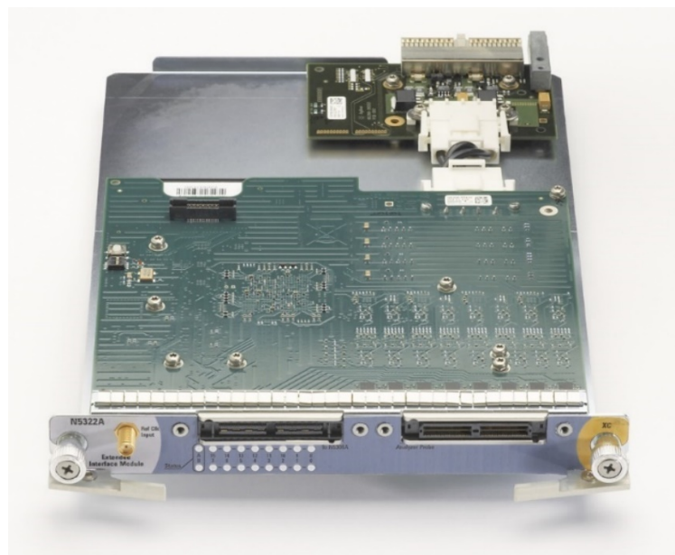
Figure 6. Extended interface module.
