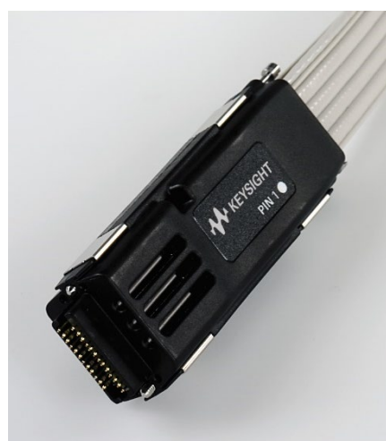
Figure 14. Half size mid-bus probe head.
