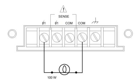
Make sure that the unit is turned off, and make the following connections to the output.
