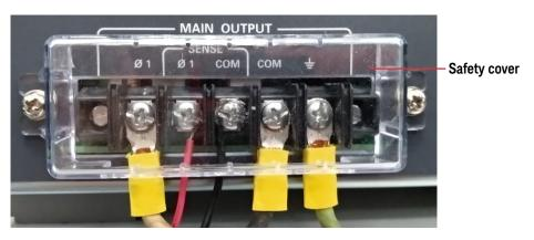
Figure 2-5 Output connections safety cover
