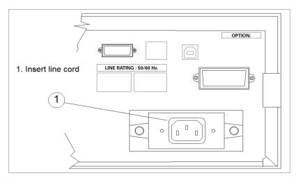
Figure 2-2 Connecting the power cord (6811C)
