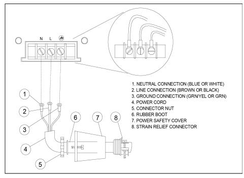
Figure E-4 Line connections
