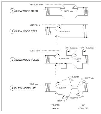
Figure 4-8 Programming slew rates
