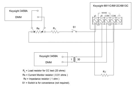
Figure B-1 Verification and calibration test setup
