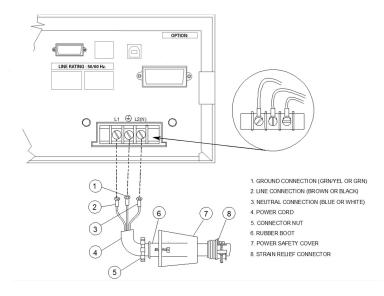
Figure 2-3 Connecting the power cord (6812C and 6813C)
