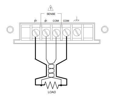
Figure 2-6 Remote sense connections
