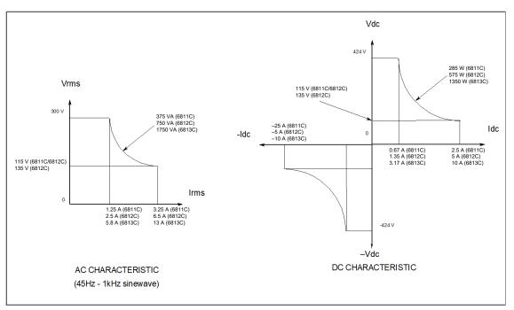
Figure 1-2 Steady-state output characteristic (in real-time mode)
