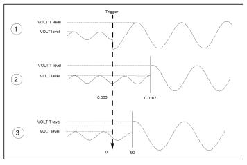
Figure 4-7 Trigger delays and phase synchronization
