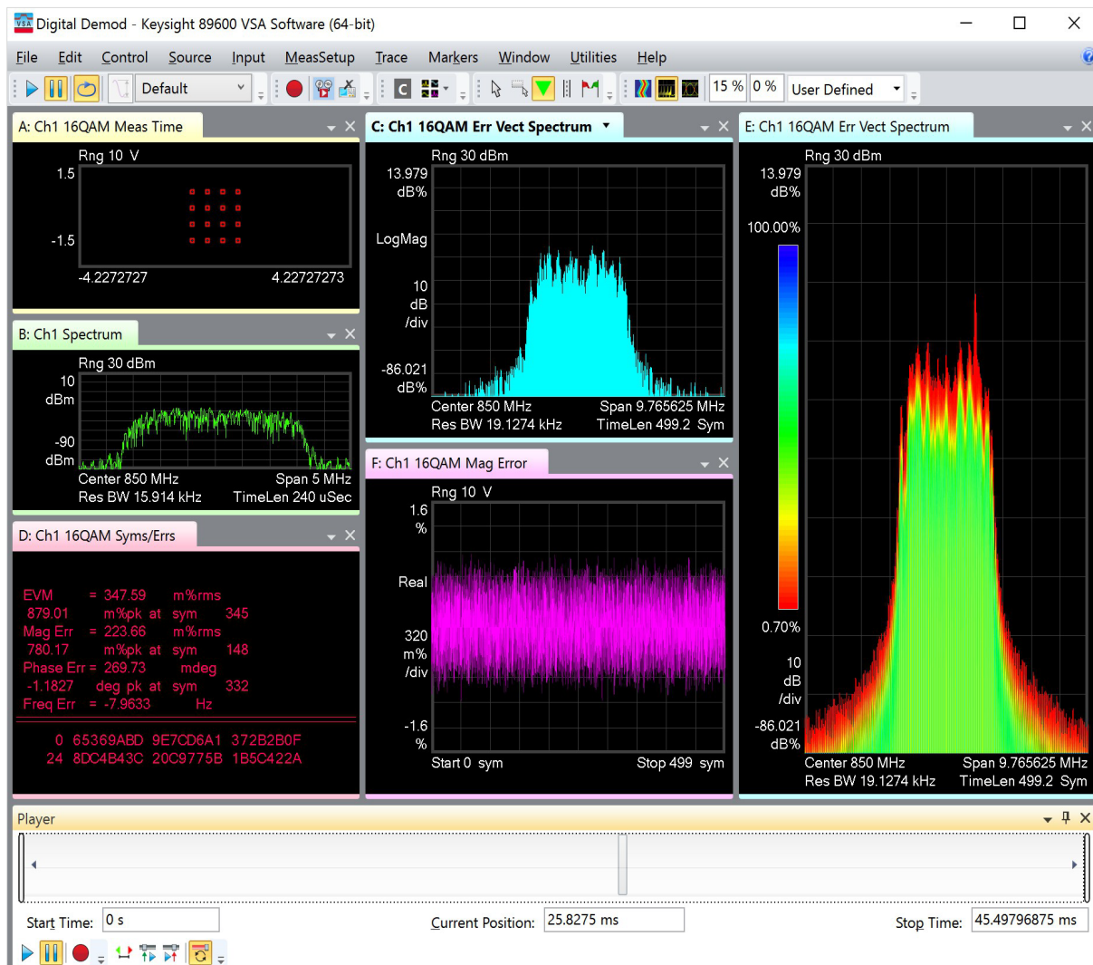
Figure 6. Save a signal and re-analyze it later with the Option AYA tools. Here, the spectrum and constellation appear to be fine. Even the EVM spectrum (trace C) is fine. But the cumulative history display of the EVM spectrum (trace E), which can highlight signal performance over > 500 hours, detects a transient error.
