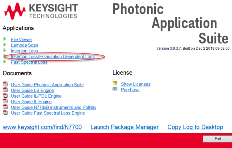
Figure 8 The Launch Pad gives you access to the installed components. Click on “Insertion Loss / Polarization Dependent Loss” to start the IL / PDL Engine.
