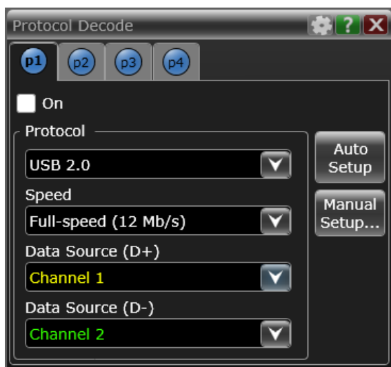
Figure 1. USB full-speed protocol decode setup window.
