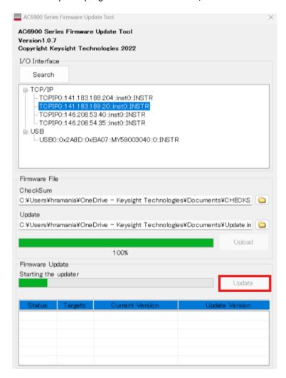
7. Once "Firmware update" progress bar reaches 100%, the "Firmware Update" will display "Firmware update was successful. Please power cycle the instrument." Click on "OK". Then, proceed to power cycle your instrument.
