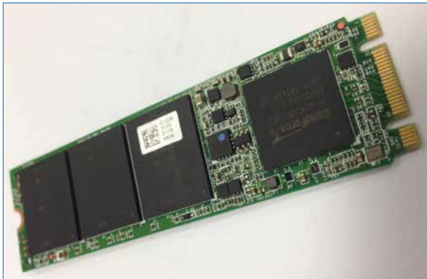
FIGURE 1. M.2 SSD for tablet and laptop PC, the smallest commercial version.
