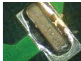
FIGURE 1. A separated connector pin post-reflow. The wetted solder suggests a plating adhesion issue.
