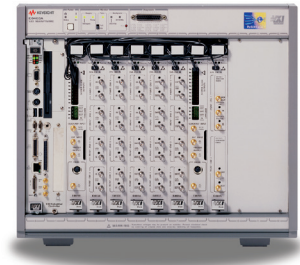
Pair a W2641A TPA with a Keysight N4903A J-BERT or 81250 ParBERT for DisplayPort sink validation.
