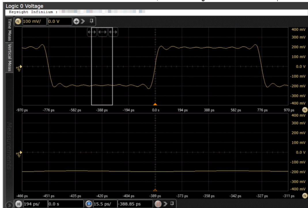
Figure 13 Reference Image for VMA for Cu (p-p) Test for Logic 0
