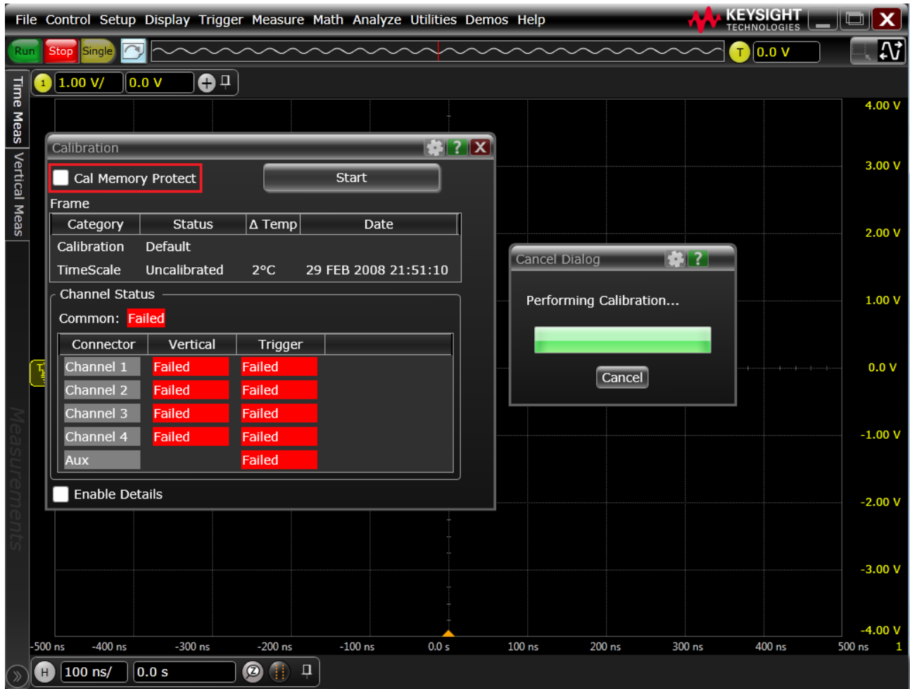
Figure 42 Clearing Cal Memory Protect and Starting Calibration
