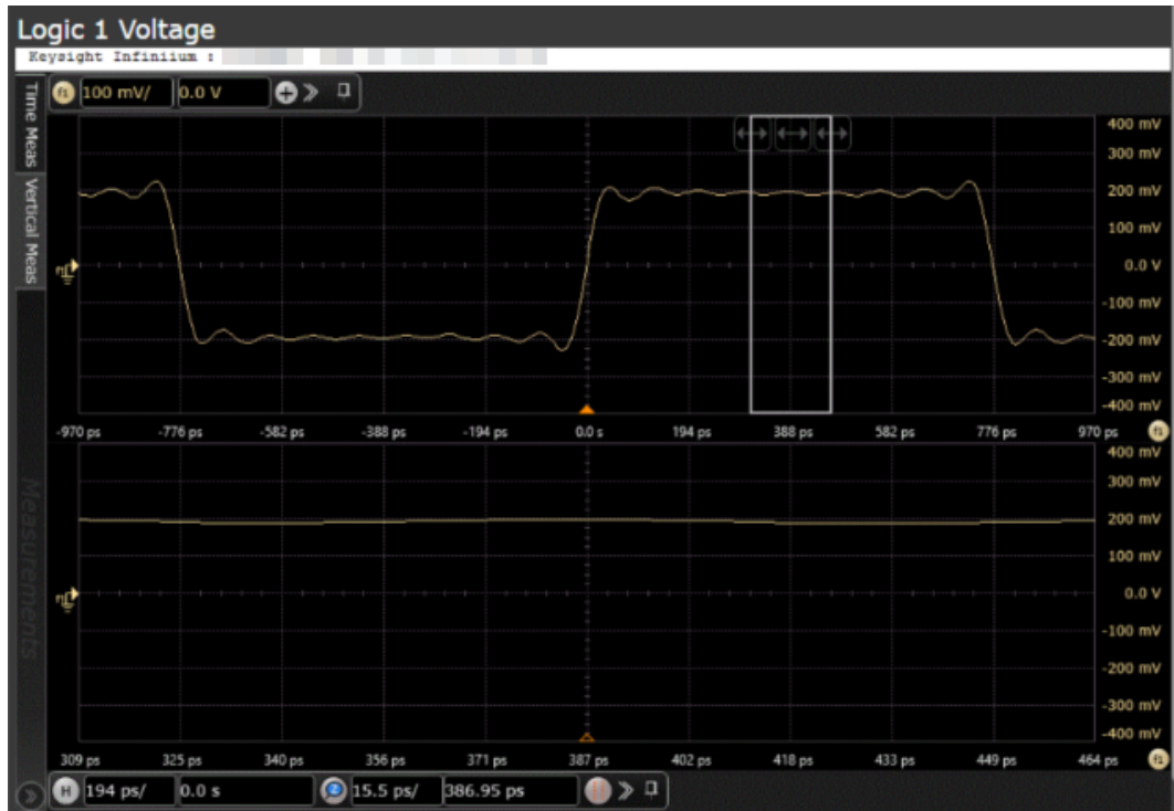
Figure 14 Reference Image for VMA for Cu (p-p) Test for Logic 1
