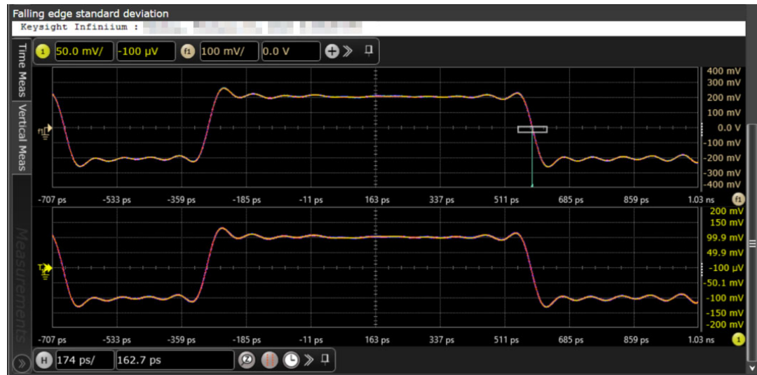
Figure 18 Reference Image for Uncorrelated Jitter (RMS) Test for Falling Edge
