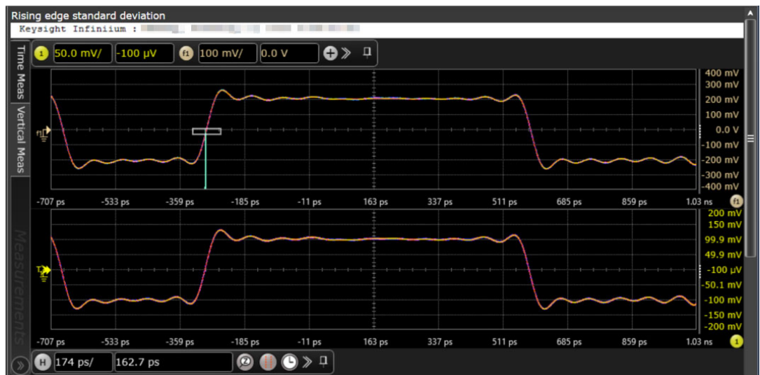
Figure 17 Reference Image for Uncorrelated Jitter (RMS) Test for Rising Edge
