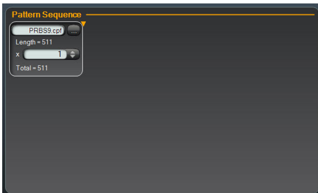
Figure 68. Loading a factory pattern
