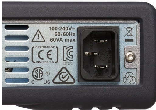
Figure 15 AC Power Requirement Markings
