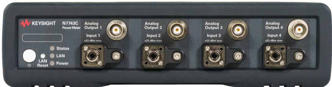
Figure 6 Front panel of the N7743C 4-port power meter
