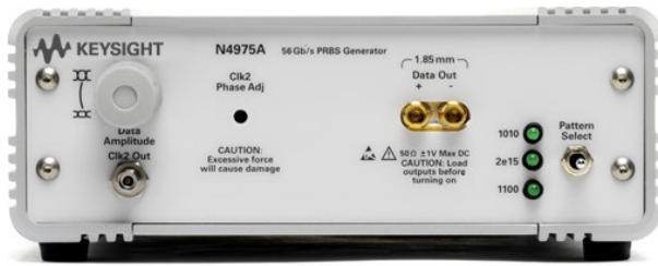
Figure 1. Front of N4975A PRBS generator 56 Gb/s. Figure 2. Back of N4975A PRBS generator 56 Gb/s.
