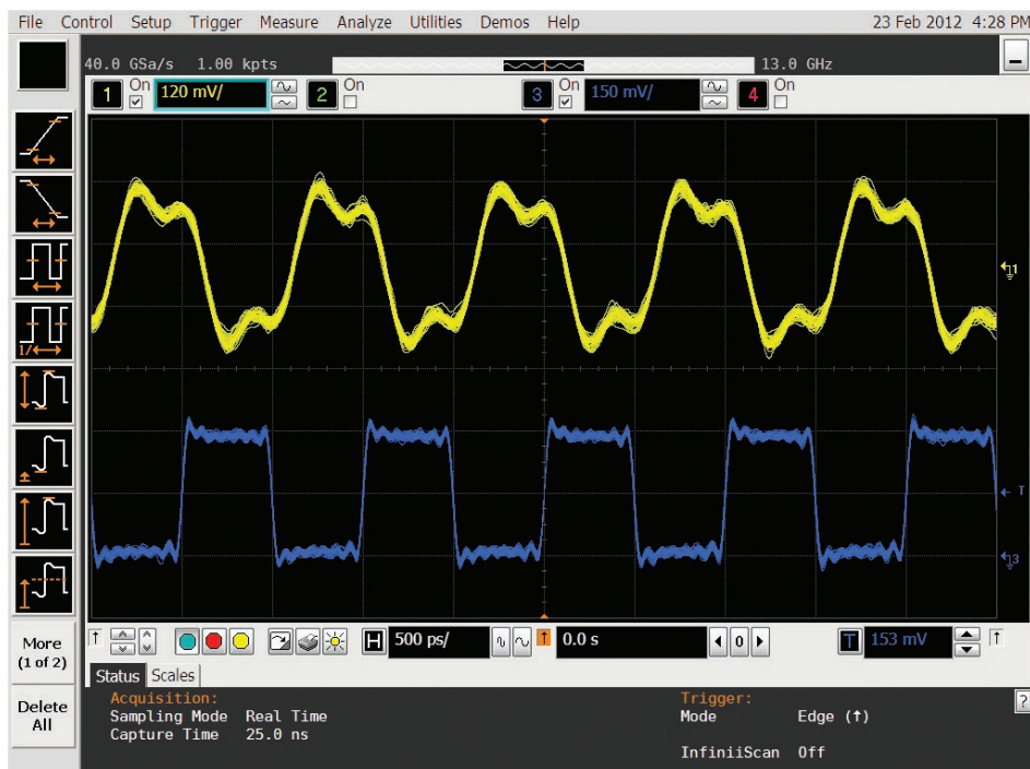
Figure 4. Time-domain waveforms measured with the Infiniium 90000 Series oscilloscope.
