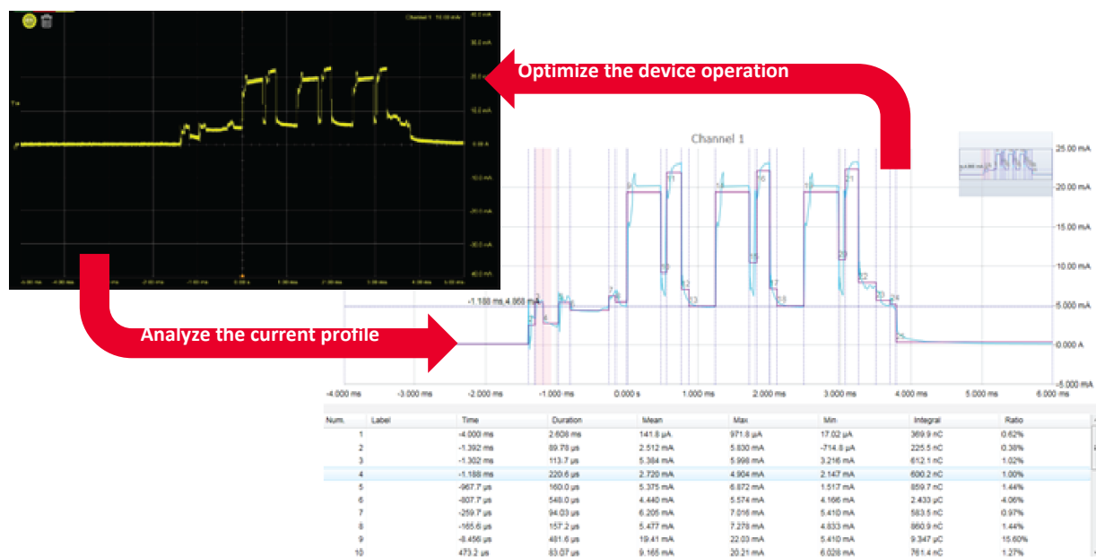
Figure 1. Automatic Current Profiler automatically adjust the time scale by the vertical level difference, instantly calculate key parameters such as average current, max/min current, accumulated charge.
