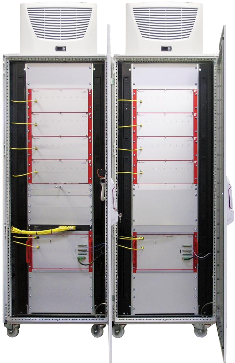
SL1007A Cell Test System – Double rack-cabinet configuration, front doors opened. Example configuration for large channel count or very high-current system.
