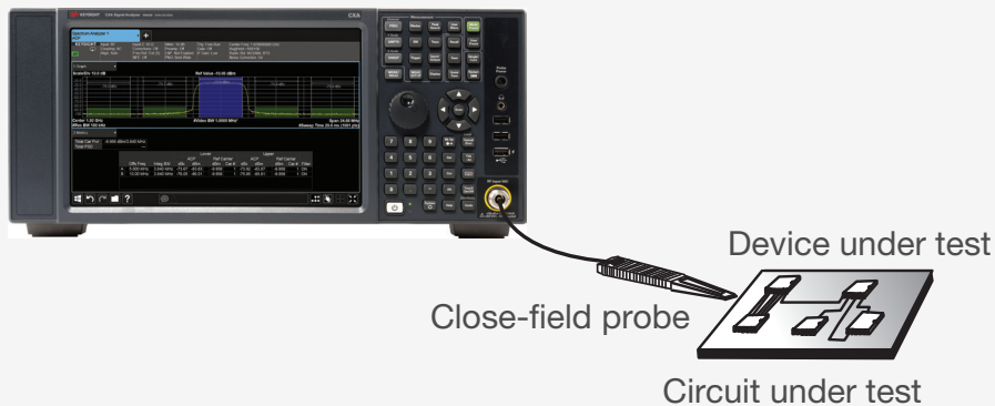
Figure 14. Diagnostics setup interconnection.
