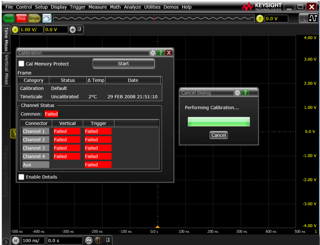
Figure 51 Clearing Cal Memory Protect and Starting Calibration
