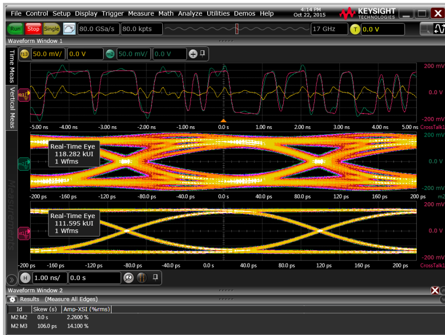
Figure 4. Before and after view of a victim waveform with FEXT. The top plot shows the victim waveform in green, the aggressor in orange, and the crosstalk removed waveform in red. The middle plot is the eye diagram of the victim with the bulging indicative of FEXT, and the bottom plot is the eye diagram of the victim after removing crosstalk.
