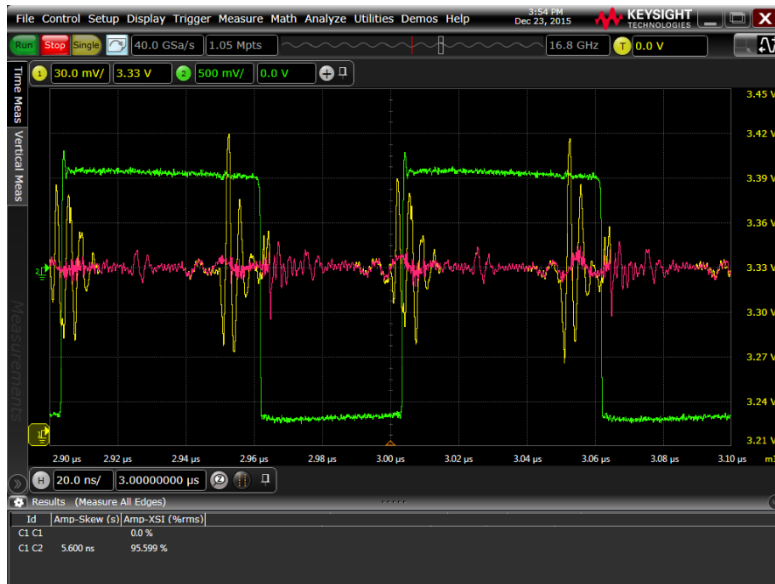
Figure 8. Example of a power supply being treated as a victim. Victim waveform (yellow), aggressor (green) and crosstalk-removed waveform (red).
