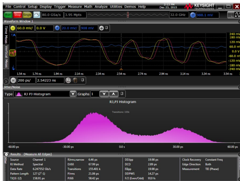
Figure 6. Jitter analysis results using EZJIT, showing the large amount of jitter in the original serial data waveform.
