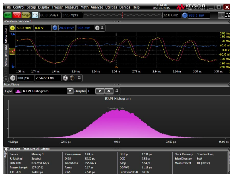
Figure 7. Jitter analysis results using EZJIT, demonstrating the improvement in jitter statistics after removing the jitter generated by the power supply.
