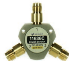
11636C DC to 50 GHz power divider
