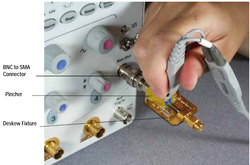
Figure 107 Browser Probe Head Calibration Connection Example
