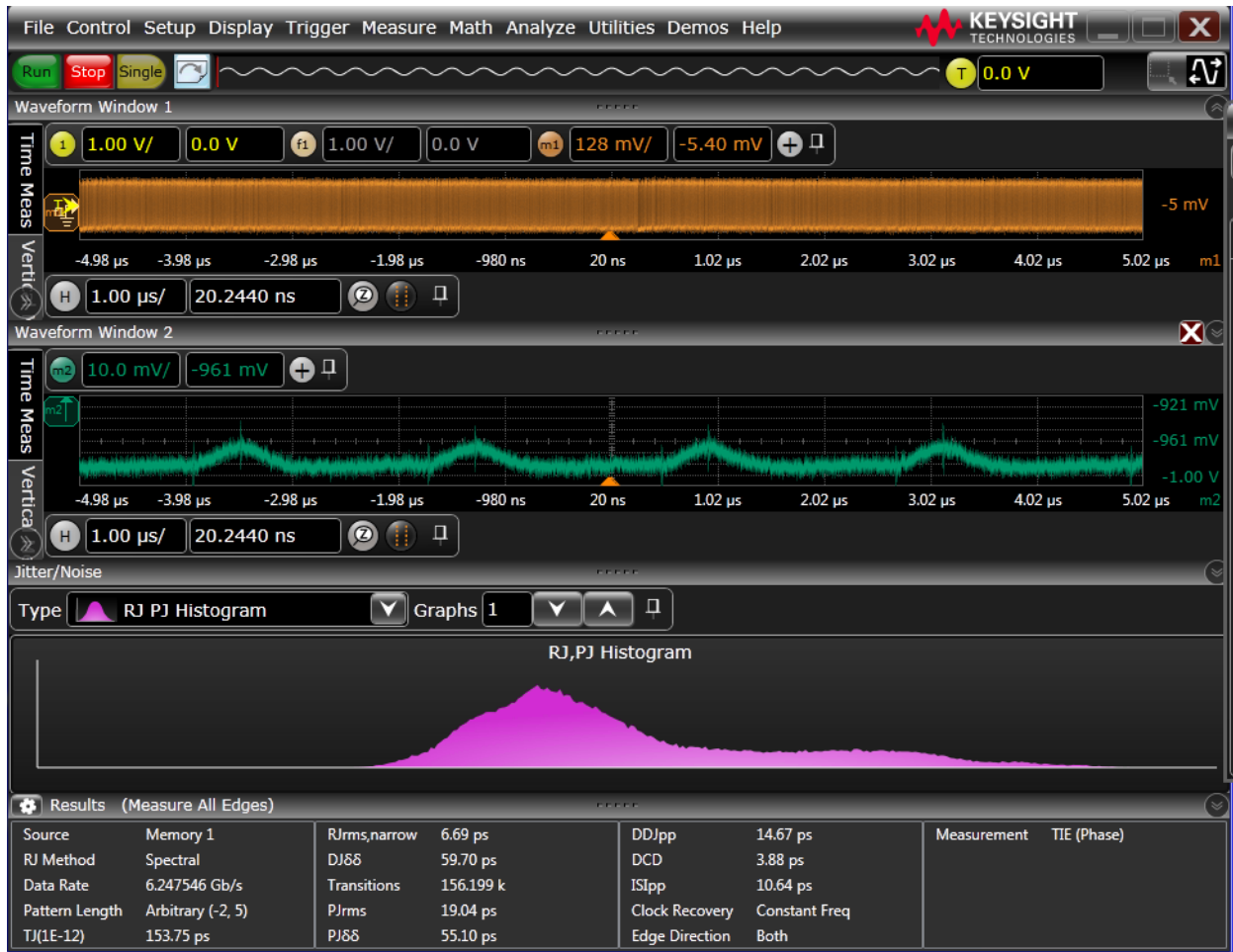
Figure 18 Jitter analysis results using EZJIT, showing the large amount of jitter in the original waveform
