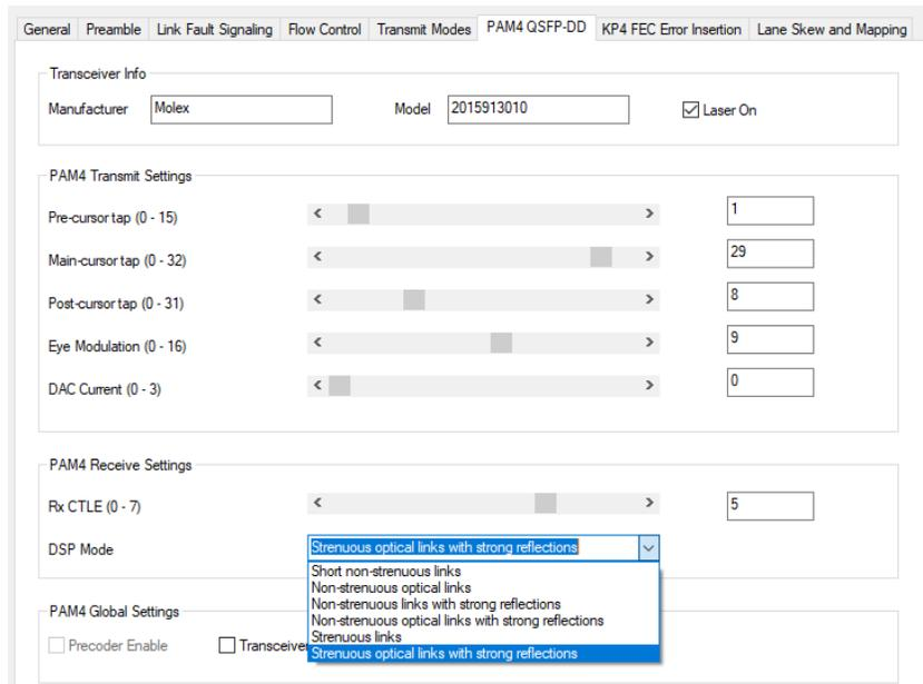
Figure 7: IxExplorer PAM4 QSFP-DD optical settings for “Strenuous optical links with strong reflections”
