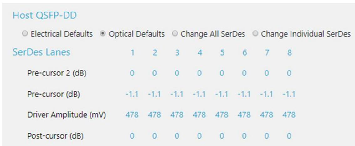
Figure 1: KiOS Host QSFP-DD settings screen for optical transceiver *Optical Defaults*
