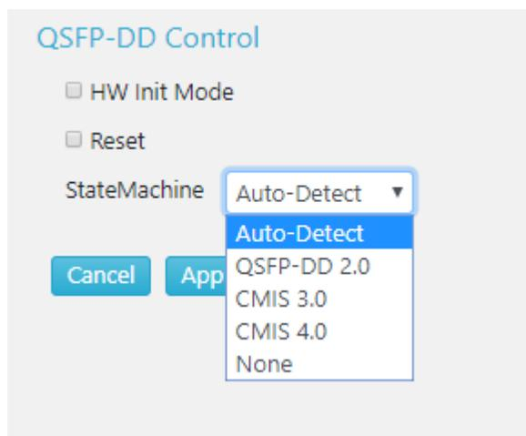
Figure 3: The KiOS QSFP-DD Control State Machine default is set to *Auto-Detect* the CMIS
