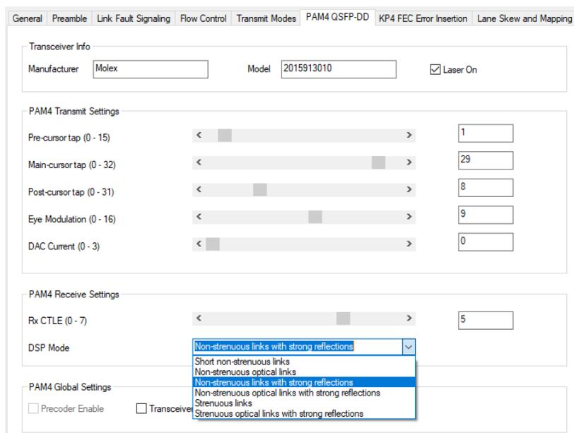
Figure 6: IxExplorer PAM4 QSFP-DD optical settings for "Non-strenuous links with strong reflections"
