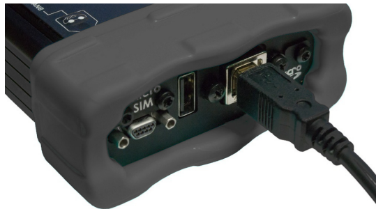
Figure 4-7 Connecting the USB Cable to the AP1200A
