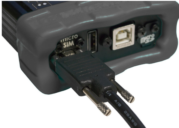
Figure 4-6 Connecting the \mu DB-9 Cable Connector to the AP1200A
