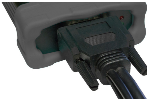
Figure 4-4 Connecting the HD-26 Cable Connector to the AP1200A
