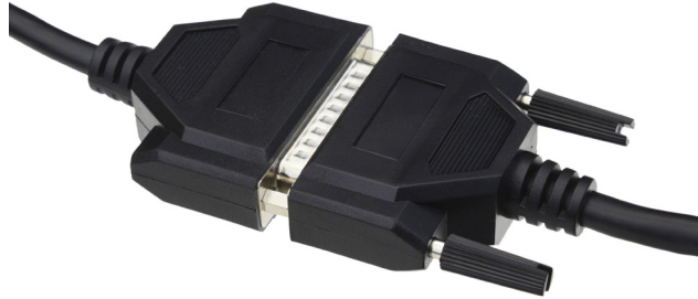
Figure 4-5 Attaching the DB-25 Connector of an OBD Cable to the DB-25 on the AP1200A Ethernet Cable Adapter
