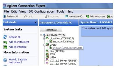
8. To the left is a Task Guide pane. Select "Send Commands to this Instrument." If you don't see this pane, select: View > Task Guide. A command window should appear as shown in Figure 7 below.
