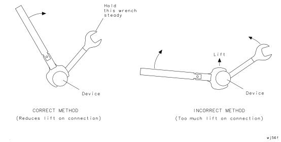
4. Hold the torque wrench lightly, at the end of the handle only (beyond the groove). See Figure 3-3.
