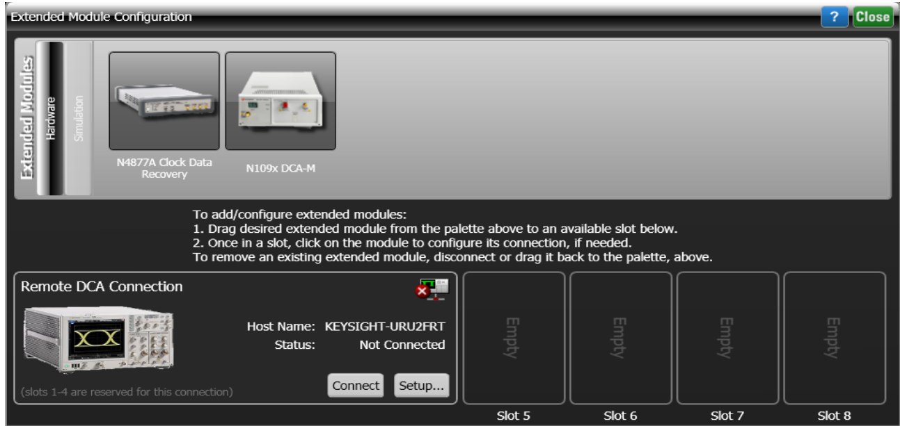
Figure 48 Extended Module Configuration dialog box for connecting N1010A FlexDCA to 86100D
