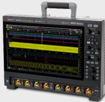
1. Combined flexible memory on the MXR shares 1.6 Gpts of memory between 4 channels. This means on a 4-channel model, you can have one channel with 1.6 Gpts, two channels with 800 Mpts, three channels with 533 Mpts memory, or 400 Mpts on four channels. This same logic applies to channels 5-8 on 8 channel models—resulting in two channels with 1.6 Gpts, four channels with 800 Mpts, six channels with 533 Mpts memory, or eight channels with 400 Mpts.
